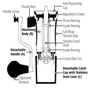
Maximum Dose: 30 grams Minimum Grind Adjustment: .02mm
